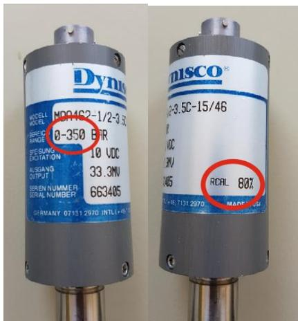
In the example, the sensor has a measuring range of 350bar as well as an integrated calibration unit at 80%.
